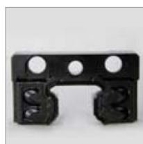
End seal in good condition
